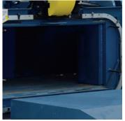
Multi-purpose door can serve as a bale separator, bale release, or bale clamp. It also allows for variable bale
