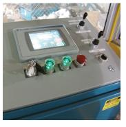
Color touchscreen operator interface PLC programmable controller features automatic and manual controls, diagnostics and bale set-up functions. Available with multi-language function.
