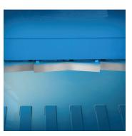
The **Galaxy** 2R wide-model ram shear blade is replaceable and reversible. The body shear blade is serrated, adjustable, and replaceable. Replaceable 500 Brinell steel liners on the floor, sides, and platens offer superior wear resistance.
