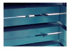
Spring-loaded container dogs are located on each side of the bale chamber to produce superior spring back control of materials being processed.
