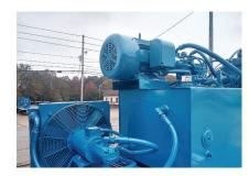
The advanced **Marathon** power pack is designed so that all of the valves are contained in a single manifold, which minimizes the number of hose connections and potential leak sources.
