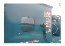
The chute feed hopper with inspection door and interlock switch will accommodate optional pneumatic, gravity, or conveyor feeding systems.
