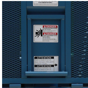
An automatic feed-gate opens at the end of each cycle as the platen is retracted.
