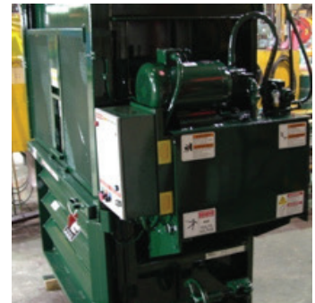
The side-mounted, self-contained power unit is convenient for maintenance and servicing. Front opening control panel eliminates the need for 48" side clearance as required by NEC standards.
