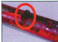
External welding on the cylinder customer modification.
