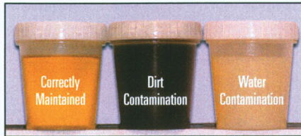
The contamination level of the oil in the hydraulic system must not exceed 18/15/13 in ISO code 4406.
