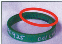
Seal damage due to paint or other unauthorized rod coating.
