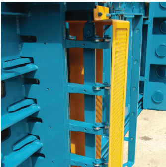
Wire positioners are on the twister cabinet side for precise twister alignment and wire pick-ups.
