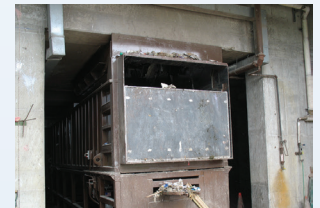
This M-1475XW Transfer Station Compactor is fed via a tipping-floor and features the Scissor trailer connection system.
