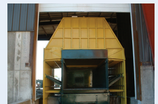
Transfer station compactors can be configured with custom hoppers and feed systems.
