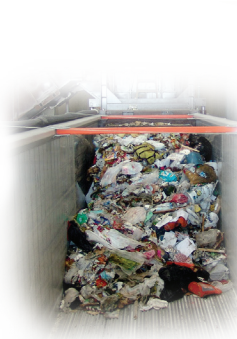
The BlokPak 3000 forms 10' (3m) logs of densely packed waste.
